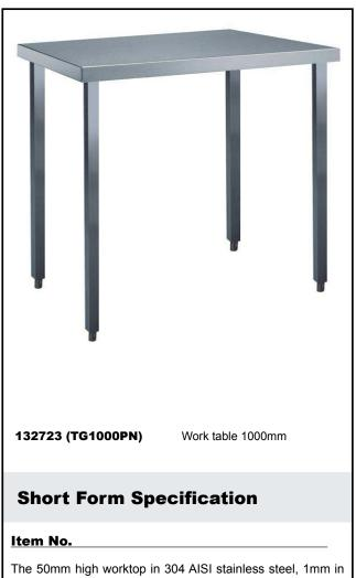
The 50mm high worktop in 304 AISI stainless steel, 1mm in thickness, has upturned edges and incorporates a layer of sound deadening, waterproof and fireproof material. Square section legs 40x40mm on 1" height-adjustable feet in 304 AISI stainless steel.
